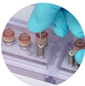
7 Screw in HUMIMIC TubeAdapters.
