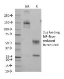
SDS-PAGE analysis of Anti-CD7 Antibody [B-F12] under non-reduced and reduced conditions; showing intact IgG and intact heavy and light chains, respectively. SDS-PAGE analysis confirms the integrity and purity of the antibody.
